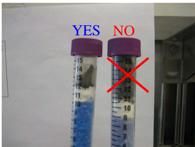
Figure 2. The scat should be loose in the tube and there should be additional space in the top of the tube as in the tube on the left. This is important in order to keep the scat dry. The tube on the right has too much scat, leading to poor DNA storage.
